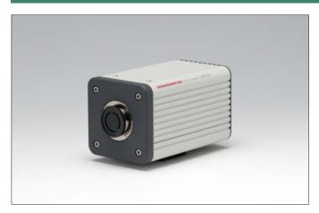
The C8000-30 employs an ultrahigh-sensitivity back-thinned CCD sensor made by Hamamatsu, which offers extremely high quantum efficiency in a wide range of UV, VIS and NIR wavelengths. The high UV sensitivity from 120 nm is useful for semiconductor mask inspection and measurement applications. Also, the high NIR sensitivity is useful for fluorescence measurement, NIR LD measurement and so on.
