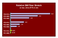
The **OPTIPHASE PZ1** is the high-speed member of our family of fiber stretchers. It is a fiber wound piezoelectric element for use in a wide range of optical interferometric measurement and sensing system applications. Typical uses include open loop demodulation, sensor simulation, variable optical delay, general purpose fiber interferometry and large angle modulation of interferometric phase.
