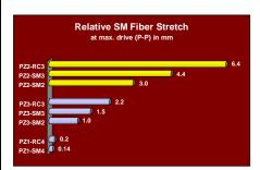
The *OPTIPHASE* PZ2 provides the most extensive stretch of our stretcher product family. It is a fiber wound piezoelectric element for use in a wide range of optical interferometric measurement and sensing system applications. Typical uses include open loop demodulation, sensor simulation, white-light scanning interferometry and large angle modulation of
