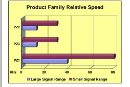
Large Signal = 70% of 1<sup>st</sup> Resonance Operation Small Signal = Frequencies extending past resonance, but at reduced modulation levels
