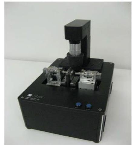
Figure 2 LFS4100 Splicing Workstation
